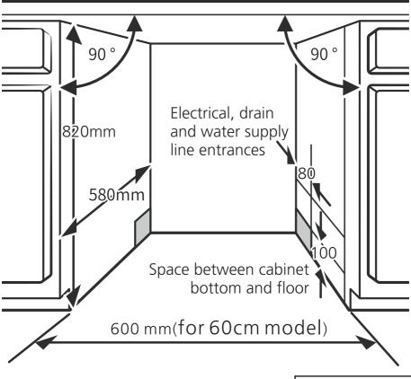
If dishwasher in installed in corner of the cabinet, make sure to allow minimum of 50mm space between opened door and cabinet.
