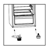
Install the adjustable feet to the right side infront of the refrigerator; mount the lower hinge subassembly to the left.
