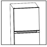
**Step 12** Install the Freezer door onto the middle hinge.
