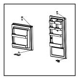
**Step 9** Remove the hinge brushing and door stop of the Refrigerator Door and the Freezer door with screwdriver, and install them to the other side of the doors.
