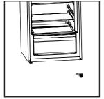
**Step 6** Remove the lower hinge with a screwdriver.
