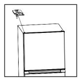
**Step 13** Use a screwdriver to mount the top hinge to the left side at the top of the refrigerator.
