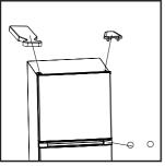
**Step 14** Mount the top hinge cover to the top hinge; mount the hinge shaft cover to the top right of the refrigerator; mount the middle beam hole cover to the right side hole of the middle beam.
