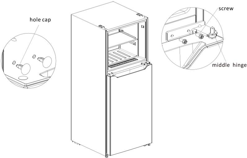
**Step 3** Remove the lower hinge assembly from lower right corner and remove the hole cap, screw cap from lower left corner; Dismantle the hinge shaft and adjustable foot and install them on the other side of lower hinge; then install the lower hinge assembly on lower left corner by fitting screws, and install the hole cap and screw cap on lower right corner.
